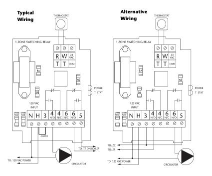
Note: When using Alternative Wiring diagram, the boiler operating control's ZC terminal will see the load of the circulator(s).
